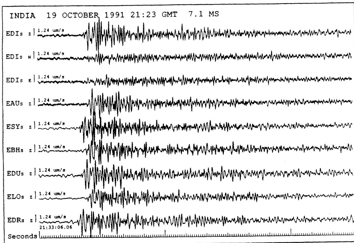
**Figure 11.** Seismograms recorded on the Lowlands network around Edinburgh, from the magnitude 7.1 MS earthquake in India on 19 October 1991. Three letter codes refer to stations listed in Annex E.
