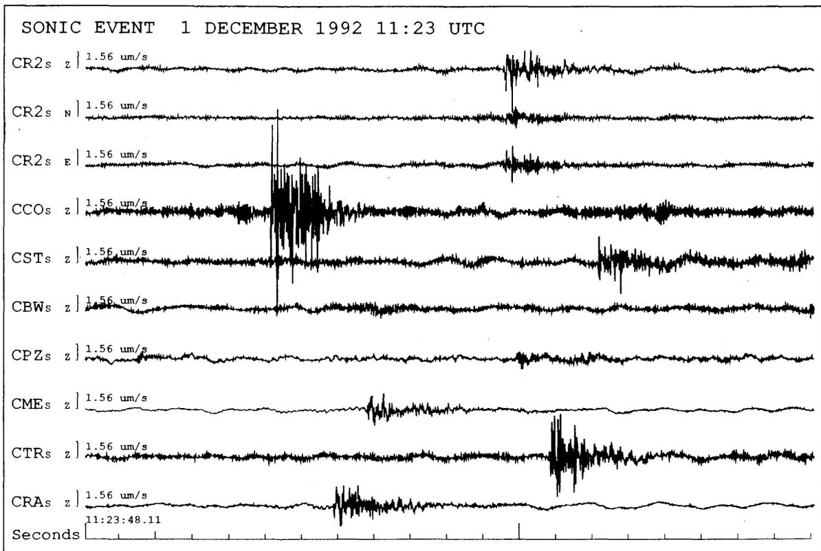
**Figure 11.** Seismograms recorded on the Cornwall network from a felt sonic event on 1 December 1992. Three letter codes refer to stations in Annex E.
