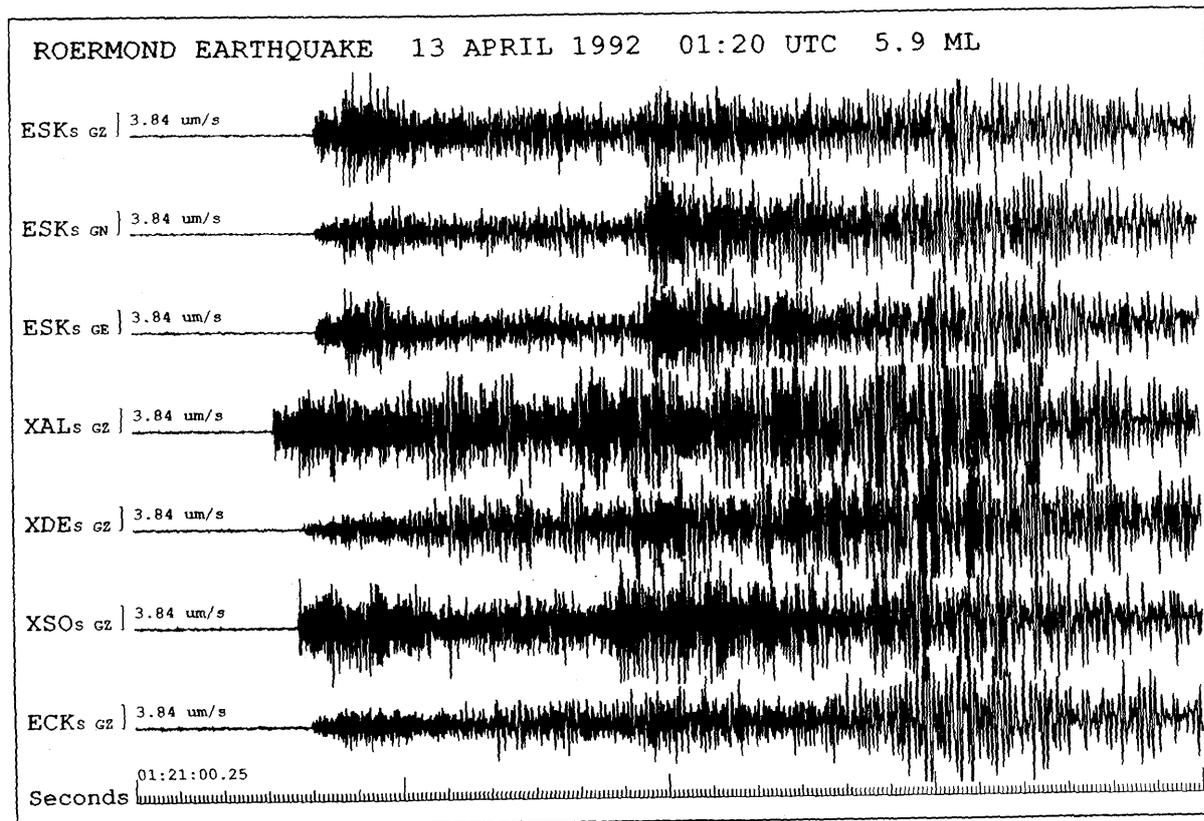
**Figure 12.** Seismograms recorded on the Eskdalemuir network from the magnitude 5.9 ML earthquake in Roermond on 13 April 1992. Three letter codes refer to stations in Annex E.
