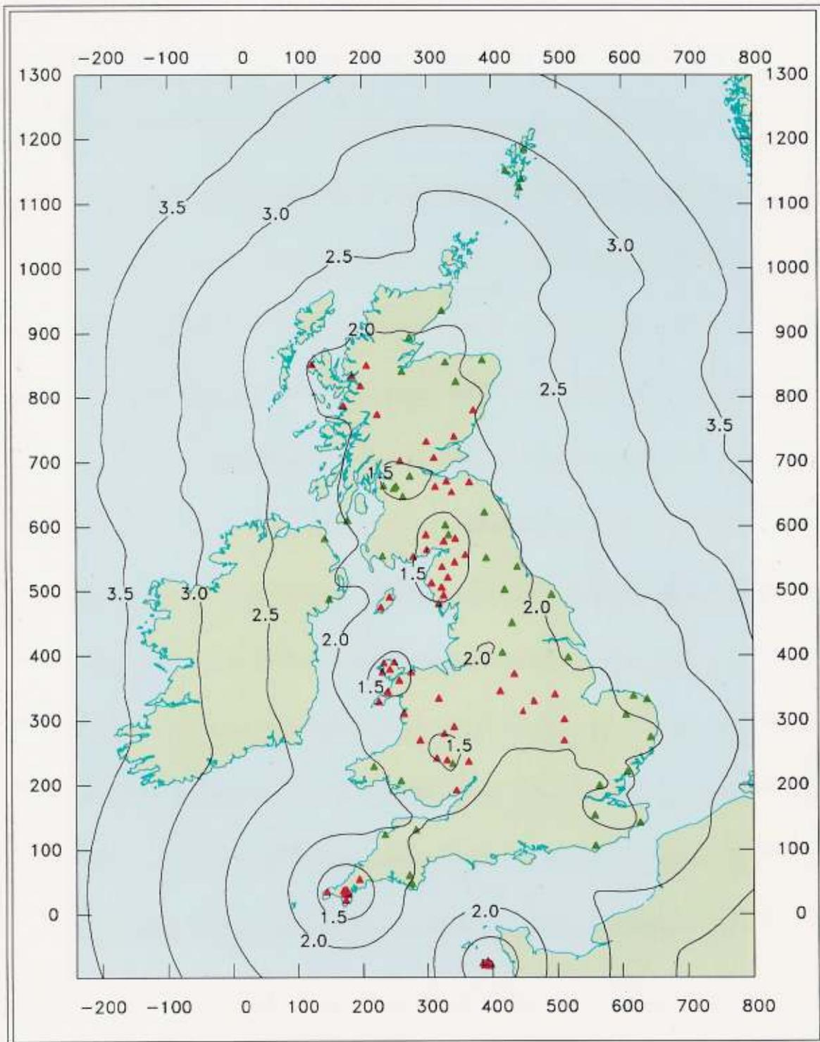
Figure 5. Earthquake identification capability. Contour values are Richter local magnitude (ML) for 20 nanometres of noise and S-wave amplitudes twice that at the fifth nearest station.
