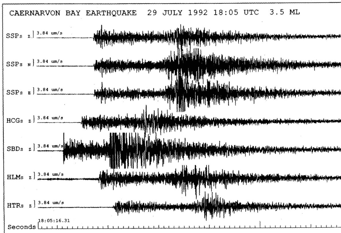
**Figure 9.** Seismograms recorded on the Hereford network from a magnitude 3.5 ML earthquake felt in the Caernarvon Bay region on 29 July 1992. Three letter codes refer to stations in Annex E.
