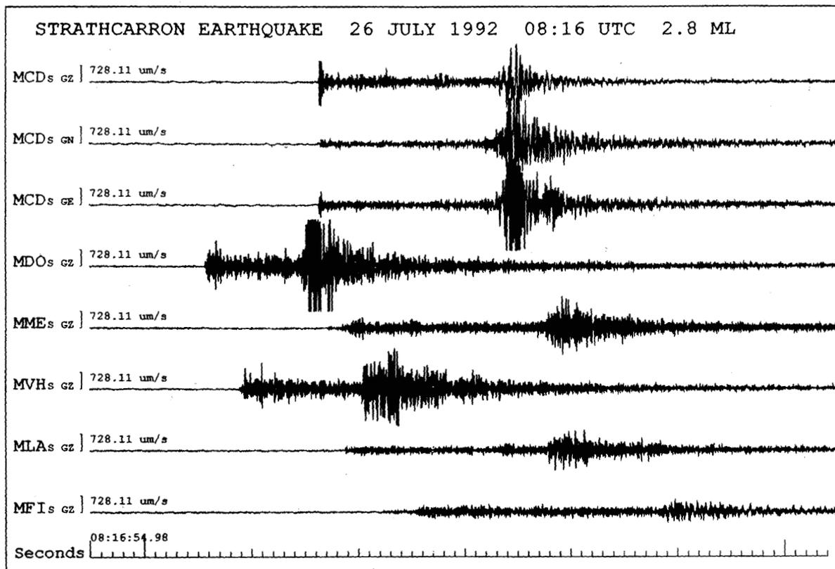
**Figure 8.** Seismograms recorded on the Moray network from a magnitude 2.8 ML earthquake felt at Strathcarron in north west Scotland on 26 July 1992. Three letter codes refer to stations in Annex E.
