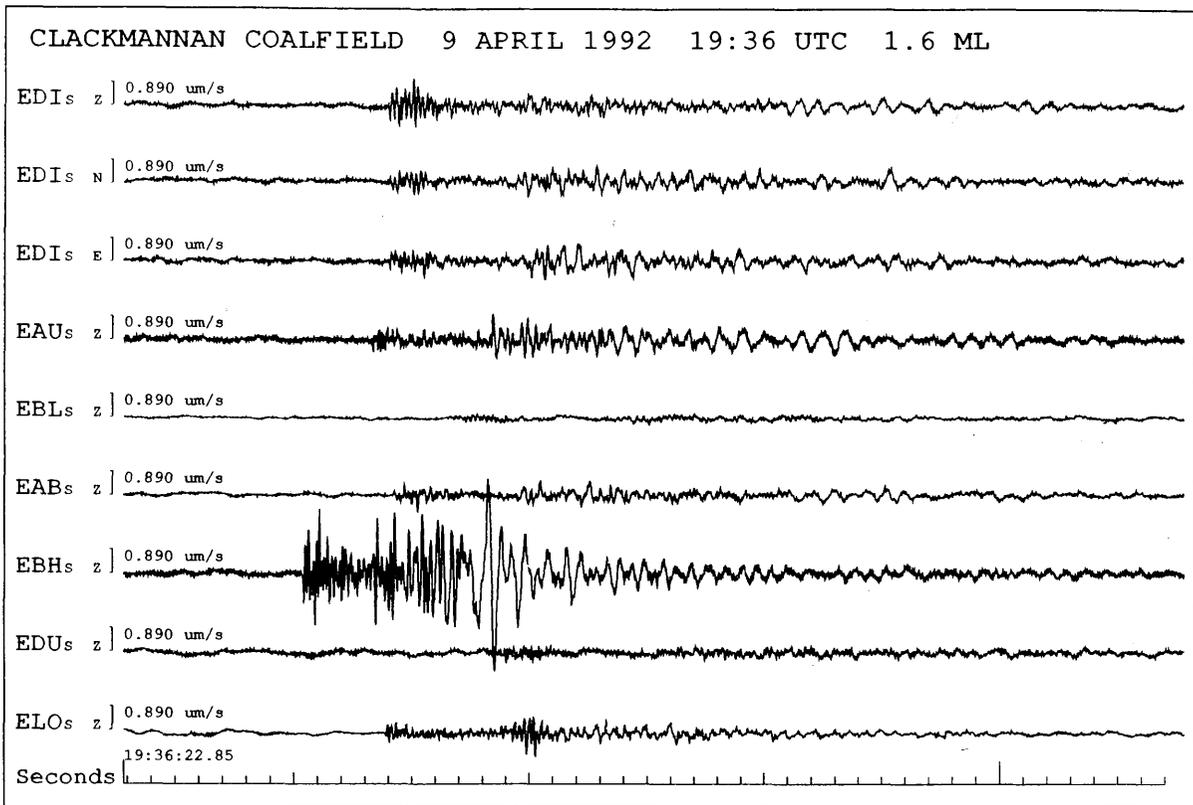
**Figure 10.** Seismograms recorded on the Lowlands network around Edinburgh from a magnitude 1.6 ML coalfield event near Clackmannan, Central Region, on 9 April 1992. Three letter codes refer to stations in Annex E.
