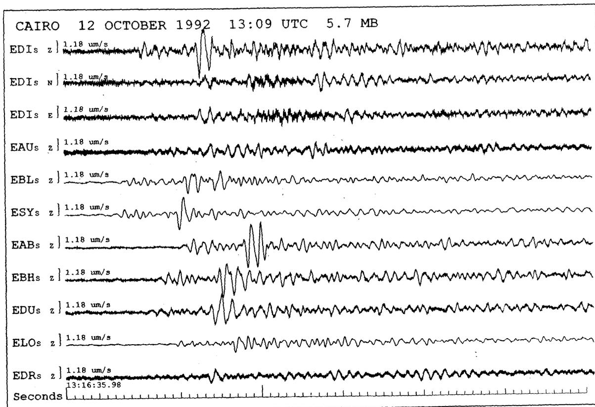
**Figure 13.** Seismograms recorded on the Lowlands network around Edinburgh from the magnitude 5.7 MB earthquake in Cairo on 12 October 1992. Three letter codes refer to stations in Annex E.
