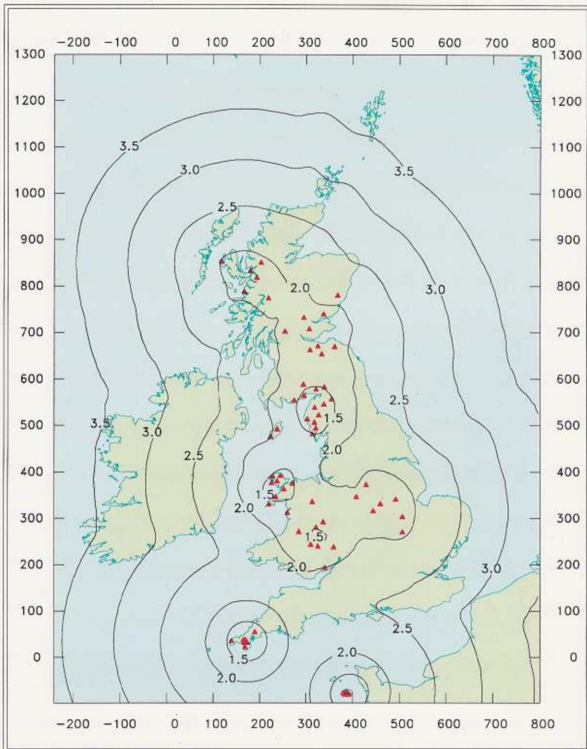
Figure 6. Detection capability of the rapid access networks. Contours show the magnitude (ML) of an earthquake which would be detected by 5 stations in the presence of 20 nanometres of background noise at 10 Hz.
